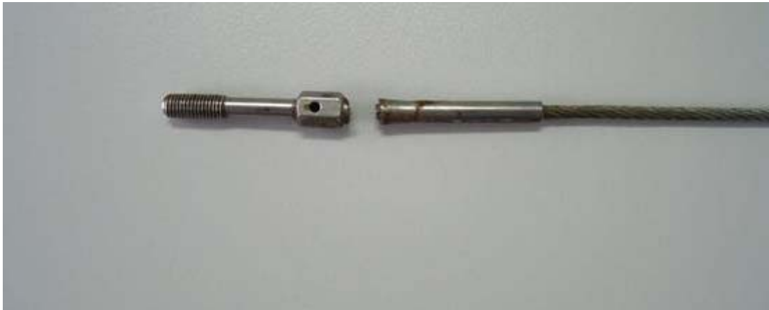
Figure 2 - Separation at swaged end of terminal
