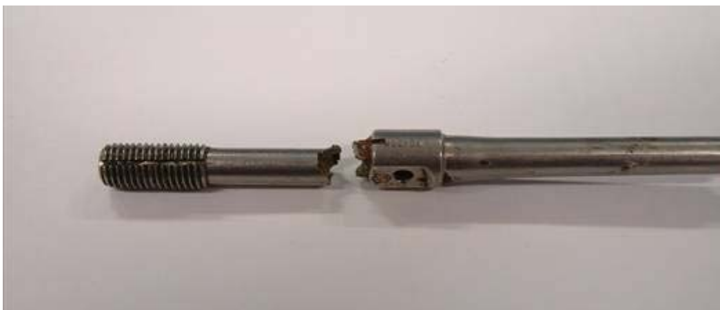
Figure 1 - Separation at threaded end of terminal
